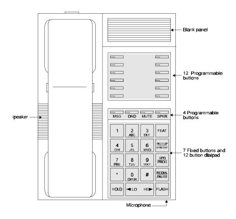
Figure 1 Four button and 16 button set faceplate
